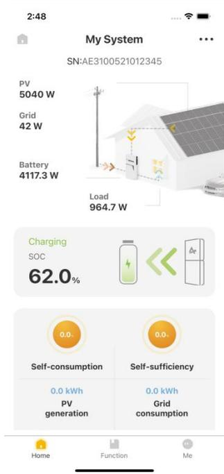
The relative value should be like this:  $Load = PV \pm GRID - Battery$
