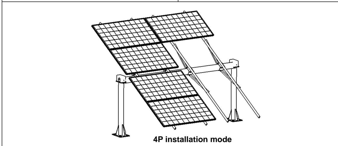
Risen module can be installed and used on the tracking system, and the installation hole position or clamp position shall be selected according to the design of the support system. Please refer to section 8.1 ,8.2and 8.3 for details,
