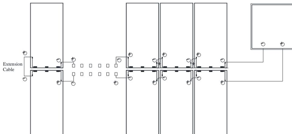
**Fig. 9-1 Split J-Box at module side position for vertical direction**
