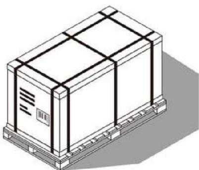
Packaged products can be shipped by land, sea, or air. During transportation, please fix the packing box on the transport platform to ensure that the packing will not roll over. No more than 2 layers by truck normally.
