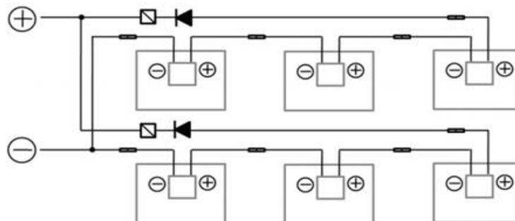
Fig. 9-3 Parallel-series Connection
