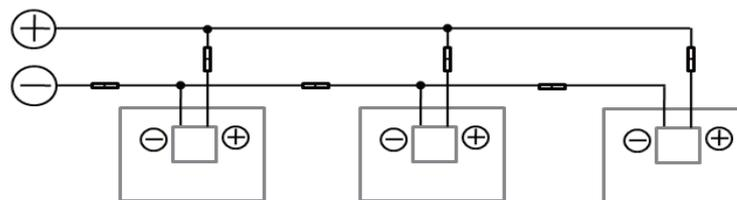
Fig. 9-2 Parallel Connection
