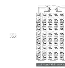
Module current output is 8.7A, current mismatch in series is **0.3A**.
